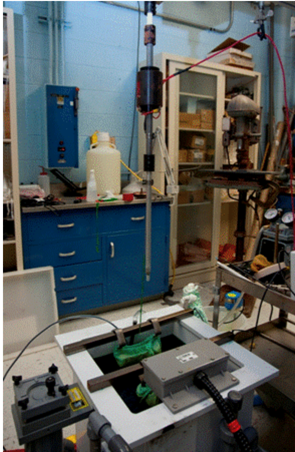
Fig. 8: Nickel electroplating bath for plating uranium metal foils
